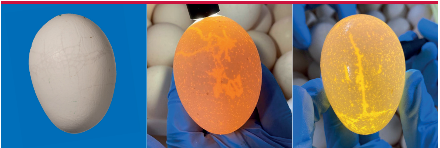
FIGURE 1: Examples of a body-checked egg (left) and illuminated hairline cracks (right).
