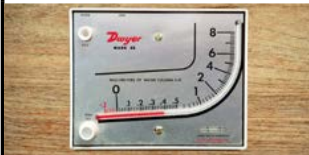
Figure 6.9 A manometer used to monitor air pressure within the house (the reading given is equivalent to 3.8 mm [0.15 in] of water column [37.5 Pa]).
